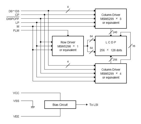
The LCD module needs two power sources:  $V_{CC}$  for logic and  $V_{ee}$  for LCD drive. (See also the above figure.)
