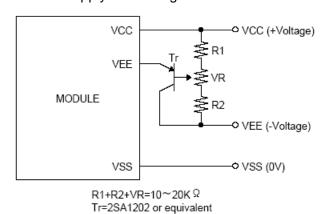
\*VDD-V0: Liquid Crystal driving voltage VR:  $10K \Omega \sim 20K \Omega$
